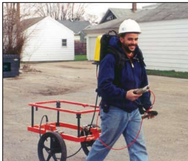
No matter how deep our clients' environmental concerns are, we are able to detect, define and eliminate them so they enjoy liability free prosperous business. Above, a SER 90 , Inc. team member conducts an EM-61 survey
