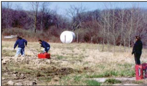
Our professionals delineated waste limits at municipal and hazardous waste landfill using non-intrusive geophysical techniques.
