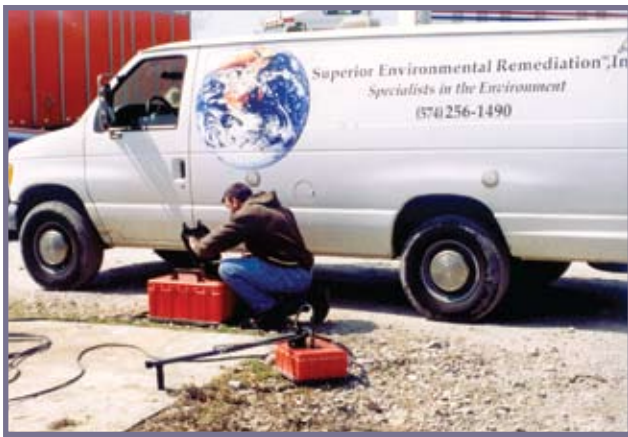
SER 90 , Inc. team member sets up instrumentation for seismic survey at a client's site.
